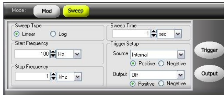
Figure 2-28 Panel view of sweep
