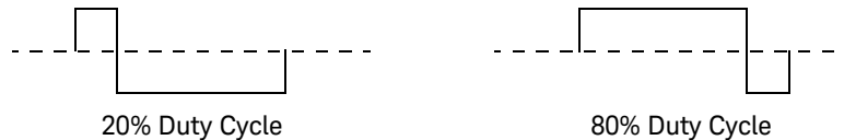
Figure 2-7 Square wave duty cycles
